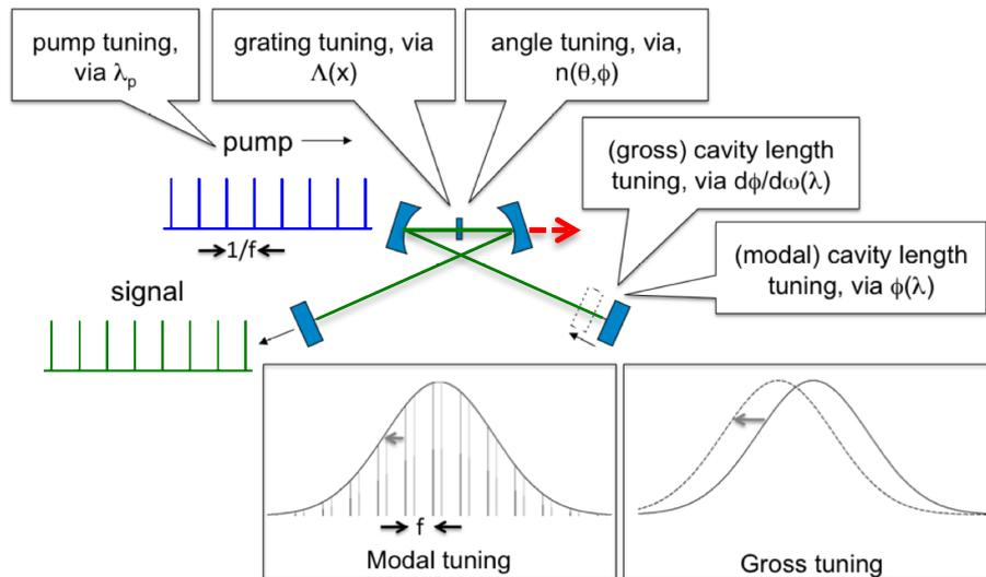
**Fig. 2.** Layout and tuning implementation in a synchronously pumped optical parametric oscillator
