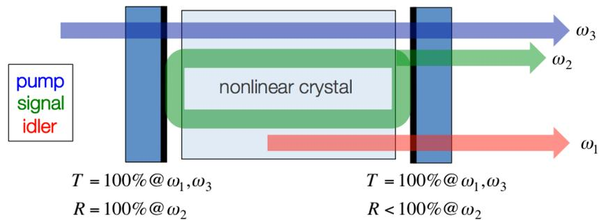
**Fig. 1.** Schematic representation of an optical parametric oscillator.
