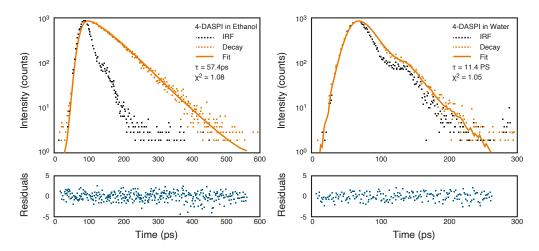
FIGURE 5. Fluorescence decays of 4-DASPI in (a) ethanol and (b) water measured using TCSPC.
