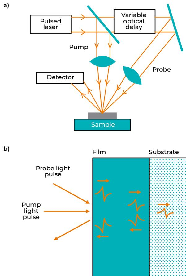
**FIGURE 1.** a) Block diagram of typical setup. b) A strain pulse is generated by the pump, is reflected at the interface between the film and the substrate, and is detected by the probe pulse when it returns to the free surface.
