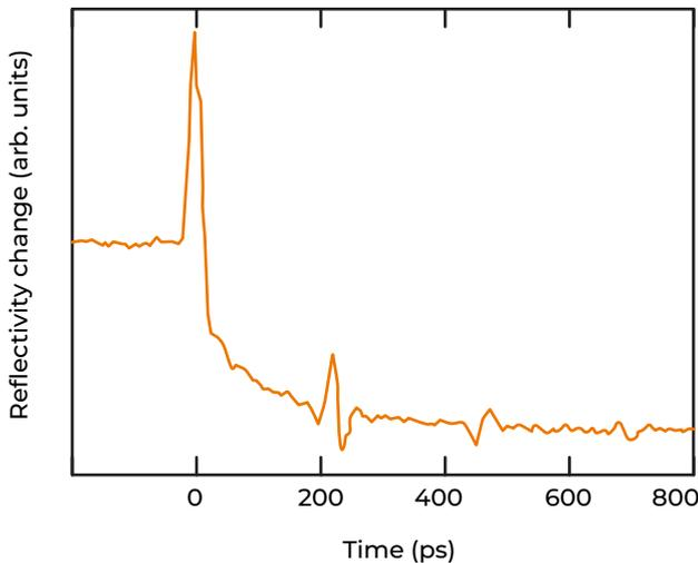
**FIGURE 2.** Example of acoustic echoes detected in a film of  $\text{As}_2\text{Te}_3$  of thickness 2200 Å.\* These echo signals can provide a high-resolution measurement of the thickness of the layer.
